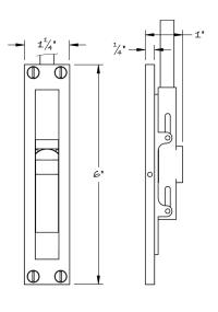
A larger version of our #4064 surface/edge bolt. Again this bolt can be mounted to the door edge or face and the rod bolt is cut to length allowing for placement anywhere vertically on the door.
