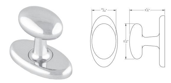
The #5004 knob with its hidden escutcheon fasteners is ideal when used as a turning piece with our mortise latches and zero flange rim latch. The piece is still based around our standard elliptical cabinet knob but its straighter shank and flush mounted base steer designers to use it in more minimal interiors.
