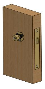
STEP 3: Drill pilot holes for the six #8 subrose mounting screws. Install the subrose mounting screws and remove the 5097 alignment tool.
