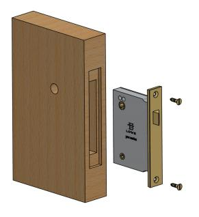
STEP 1: Instal I lockset into the door that has been mortised according to the lock template.
