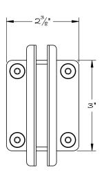
Standard shower door hinges for glass panels. These hinges can be specified for 3/8" or 1/2" thick glass.
