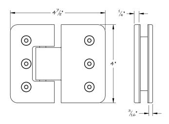
Standard shower door hinges for glass panels. These hinges can be specified for 3/8" or 1/2" thick glass.
