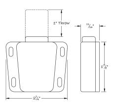
The 6094 push latch features 25 lb push force and is suitable for use on doors with a minimum thickness of 5/8".
