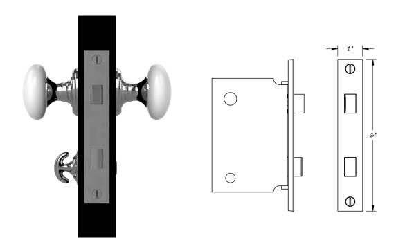
The Lowe #349 full mortise interior privacy lock is available in 2", 2–1/4", 2–1/2", and 2–3/4" backsets as standard. Custom sizes available upon request. This lock is typically used on interior doors of all sizes and can be configured at the factory to be used with knobs or levers. Supplied with strikeplate and dustbox, the faceplate is adjustable for beveled doors.
