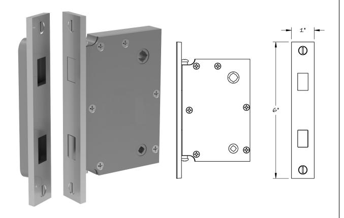
The Lowe #349M full mortise Magnetic interior privacy lock is available in 2", 2-1/4", 2-1/2", and 2-3/4" backsets as standard. Custom sizes available upon request. This lock is typically used oninterior doors of all sizes and can be configured at the factory to be used with knobs or levers.
