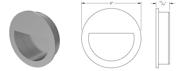
All hardware is made-to-order. Details and dimensions can be modified to suit any project.
