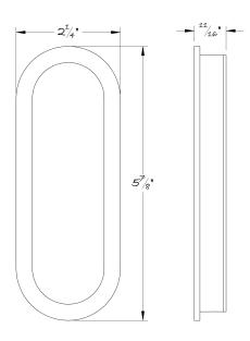
All hardware is made-to-order. Details and dimensions can be modified to suit any project.
