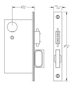
The 4182 is available in 2", 2-1/2", 2-3/4", 3-3/4", 5", and 6" backsets. The full mortise pocket door edge pull features hidden spring activated bail. Shown here in the extended position, the bail is depressed to extend or release. The 4182 features a deadbolt suitable for use with privacy and security functions and is supplied with a strikeplate and dustbox.
