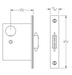
Lowe 4181 full mortise pocket door edge pull features a hidden spring activated bail, released by depressing the bail. Shown here in the extended position.
