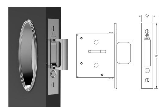
The 4200 full mortise pocket door edge pull features a spring activated bail released by a push button to pull doors from their pockets. The faceplate has an adjustable bevel.
