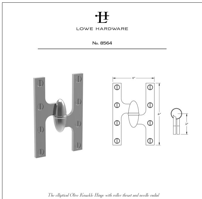
I he elliptical Olive Knuckle Hinge with roller thrust and needle radial bearings features a classic lift-off style, shown here in the 6"x4" option. All hardware is made-to-order. Details can be modified to suit any project. Available in any of our yacht quality finishes.
