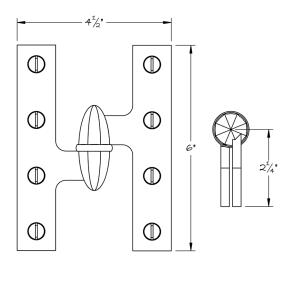
The elliptical Faceted Olive Knuckle Hinge with roller thrust and needle radial bearings features a classic lift-off style shown here in the 6" x 4.5" option.
