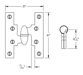
The elliptical Olive Knuckle Hinge with roller thrust and needle radial bearings features a classic lift-off style shown here in the 6" x 5" option.
