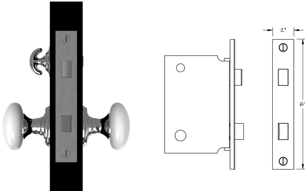
*The Lowe #349USD full mortise interior privacy lock is available in 2", 2-1/4", 2-1/2", and 2-3/4" backsets as standard. Custom sizes available upon request. This lock is typically used on interior doors of all sizes and can be configured at the factory to be used with knobs or levers. Supplied with strikeplate and dustbox, the faceplate is adjustable for beveled doors.*
