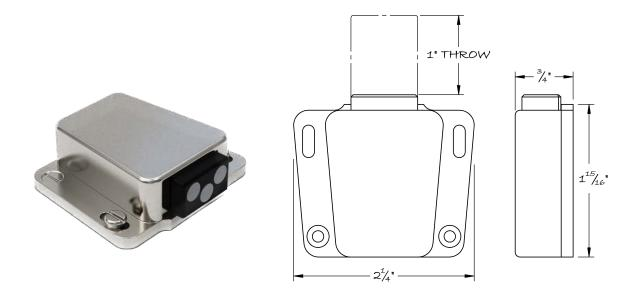
The 6094 push latch features 25 lb push force and is suitable for use on doors with a minimum thickness of 5/8".
