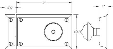
Lowe Hardware's #100 passage door rim lock combines time tested mechanical design with precision manufacturing. Upon close study of rim locks produced over the past 200 years, our engineering has led to this versatile piece machined from solid brass, bronze, or steel.
