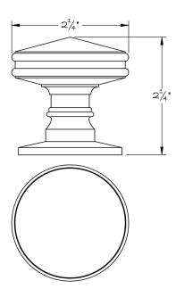
Lowe Hardware's #5022 knob comprises a head balanced by two plain astragals with a fifteen degree cone on top and a fifteen degree run on bottom leading to a coved transition to the shank. The gentle ogee curve of the rose is bound on its perimeter by a thin astragal.
