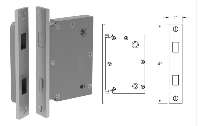
The Lowe #349M full mortise Magnetic interior privacy lock is available in 1–3/4", 2", 2–1/4", 2–1/2", and 2–3/4" backsets as standard. This lock is typically used on interior doors of all sizes and can be configured at the factory to be used with knobs or levers. Supplied with Magnetic strikeplate and dustbox, the faceplate is adjustable for beveled doors.
