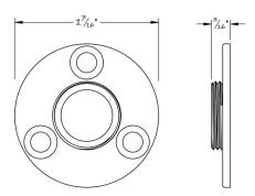
Low profile threaded subrose for use with all active knobs and levers.
