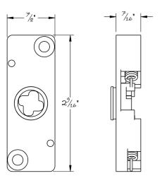
The Lowe 1599 spring assist mounts to the back of any of our escutcheon plates when needed to return heavy levers and prevent sagging. Door prep is required.
