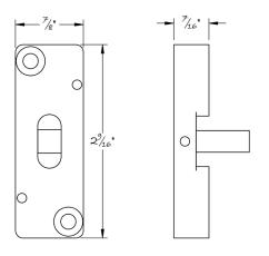
The Lowe 1599D is a dummy mount to be used on paired doors with our 1599 spring assist.
