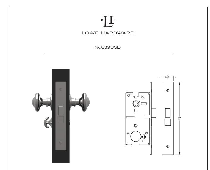
The Lowe 839USD narrow backset mortise patio lock is available in 1-1/2", 1-3/4", 2", or 2-1/4" backsets. The 839USD is typically used to secure narrow backset patio doors and other exterior doors that do not require a key. The 839USD features 1" reinforced deadbolt, full egress functionality and can also be used where a narrow backset privacy with egress function is needed.
