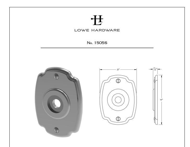
Part of Lowe Hardware's arts and crafts suite, the #1505s escutcheon plate features cloudlift details on its top and bottom. The ovolo edge molding leads to a step before the plate's flat faces. Hand hammering on this face is available upon request. The plate can be machined for use with American or European locks, latches, screen door hardware, or simply as a push plate. Projection is 3/8'.
