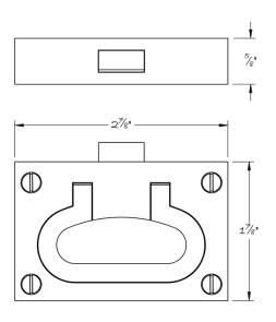
The No. 1086 Pull Latch is Lowe Hardware's refined version of a classic marine D handle slam latch.
