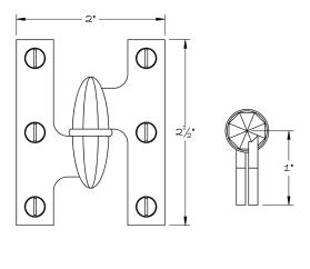
The elliptical Faceted Olive Knuckle Hinge with roller thrust and needle radial bearings features a classic lift-off style shown here in the 2.5" x 2" option.
