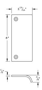
The No. 3089 bent edge pull, is available for 2-1/4" and 1-3/4" thick doors and manufactured to requested custom lengths.
