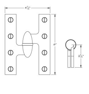
The elliptical Olive Knuckle Hinge, with roller thrust and needle radial bearings, features a classic lift-off style shown here in the 6" x 4.5" option.
