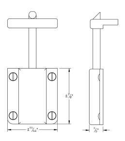
Based on the popular #1002 rim latch, the #1080 drawer latch incorporates a 1/4" diameter rod as a latching tongue. This can be cut to length depending on the drawer height.
