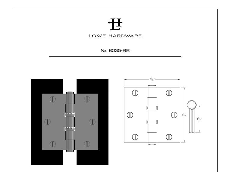
Full mortise, five knuckle, template butt hinge, sized 3 1/2" by 3 1/2", featuring two ball bearings. Lowe Hardware's butt hinges are made of the highest quality architectural brass extrusions with removable stainless steel pins. See our finials product sheet for trim options. Available in all of our yacht quality finishes.
