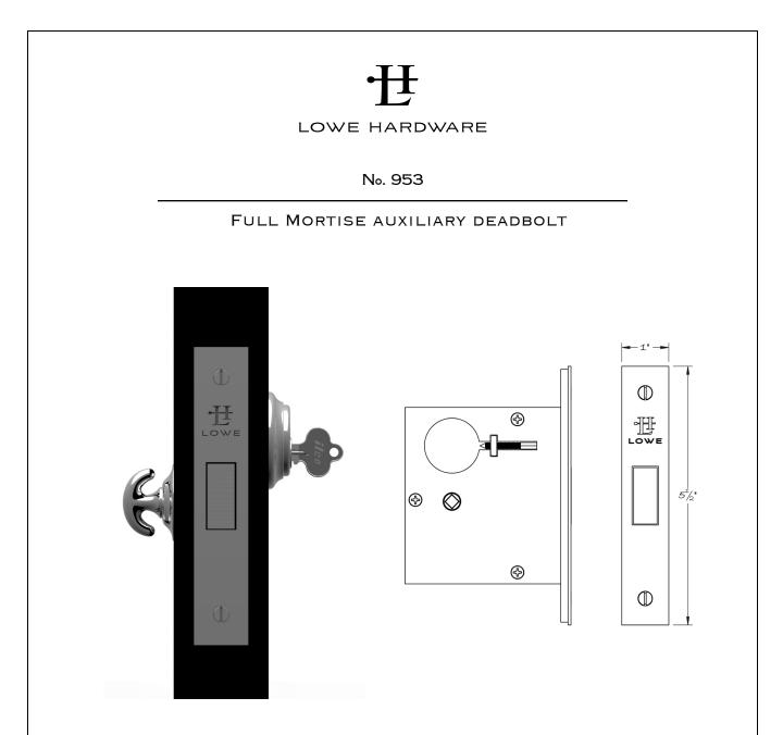
The Lowe 953 full mortise auxiliary deadbolt is available in 2-1/2", 2-3/4", 3-3/4", 5", or 6" backsets. The 953 can be used as an additional auxiliary deadbolt on exterior doors where additional security is desired, or on interior doors for both privacy and security. The lock can be configured to work with mortise cylinders, thumbturns, or emergency release trim. It is supplied with a strikeplate and stamped metal dustbox, and the faceplate has an adjustable bevel. Available in all finishes.
