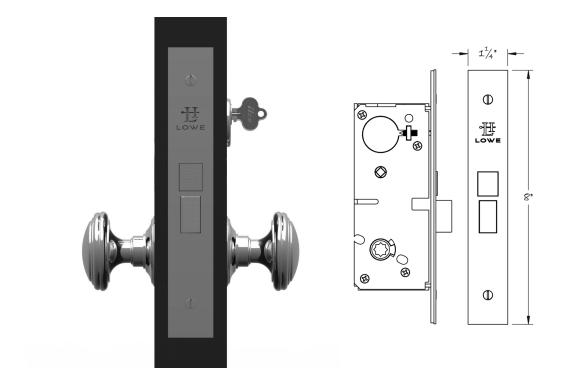
The Lowe 559 light duty, narrow backset mortise storeroom lock is available with a 1–1/4" backset. Typically used as a storeroom lock, from the outside the 559 maintains a locked position always requiring a key to enter. From the inside free egress is always available. It is supplied with a strikeplate and stamped metal dustbox, and the faceplate has an adjustable bevel.
