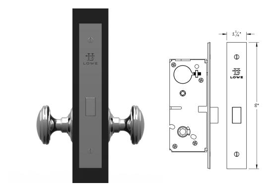
The Lowe 525 light duty, narrow backset mortise passage lock is available with a 1–1/4" backset. The 525 is typically used to on passage doors that require a narrow backset lock. It is supplied with a strikeplate and stampedmetal dustbox, and the faceplate has an adjustable bevel.
