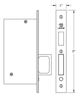
The 4203 full mortise combination pocket door edge pull and strike features a spring activated bail released by a push button to pull doors from their pockets.
