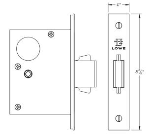
The 4201 full mortise pocket door auxiliary deadbolt is available in 2", 2–1/2", 2–3/4", 3–3/4", 5", and 6" backsets. Featuring a deadbolt suitable for use with privacy and security functions, the lock is supplied with a strikeplate and stamped metal dustbox,
