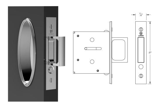
The Lowe No. 4200 full mortise pocket door edge pull features a spring activated bail released by a push button to pull doors from their pockets.
