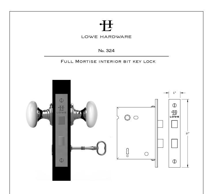
The Lowe 324 full mortise interior bit key lock is available in 2–1/2" or 2–3/4" backsets. The 324 is typically used on interior privacy doors of all sizes where the use of a bit key is desired. The lock can be configured at the factory to be used with knobs or levers. It is supplied with a strikeplate and stamped metal dustbox, and the faceplate has an adjustable bevel. Spacing between the handle and bit key is 2–7/8". Available in all finishes.
