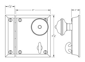
Lowe Hardware"s #101 key locking rim lock combines time tested mechanical design with precision manufacturing. Upon close study of rim locks produced over the past 200 years, our engineering has led to this versatile piece machined from solid brass, bronze, or steel.
