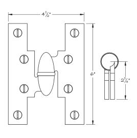
The elliptical Olive Knuckle Hinge with roller thrust and needle radial bearings features a classic lift-off style shown here in the 6" x 4.5" option.
