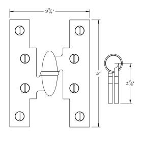
The elliptical Olive Knuckle Hinge with roller thrust and needle radial bearings features a classic lift-off style shown here in the 5" x 3.75" option.
