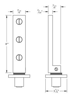
Lowe Hardware's #8010 transom pivot hinge is suitable for windows that pivot either on their vertical or horizontal axis. Constructed of solid CNC machined brass, the pin measures 5/16" in diameter.
