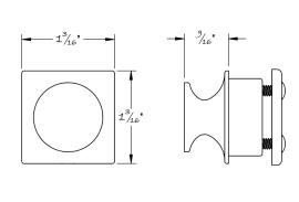
No. 7000 is designed to function as a fixed pull dummy push button.
