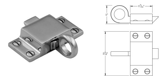
The #6300 transom catch is intended for operation by either hand or pole (using a transom hook attached to a wooden or metal pole). This catch is hot forged brass, hand polished, and has an internal spring of stainless steel. Supplied with a solid brass universal strike.
