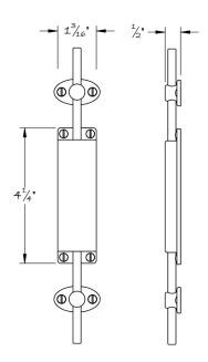
The Lowe Hardware #6099 cremone bolt for cabinet doors. Minimal in size, 1/4" diameter rods are custom cut to length and have an overall travel of 5/16", securing the door top and bottom.
