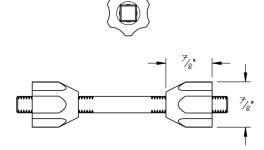
Lowe Hardware's No. 5097 alignment tool allows for perfect installation of subroses or escutcheons.
