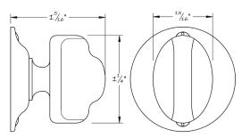
The #5084 thumbturn was originally designed for a Greene & Greene influenced interpretation of the Gamble house completed in Maine. The side profile follows the typical cloud lift pattern with flattened sides and an elliptical shape at the neck transition. Machined from solid brass, this piece can be adapted to suit any interior trim, as well as American or European lock systems.
