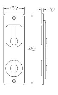
Lowe Hardware's pocket door trimsets are available as surface mounted units or with .25" radius corners for routing in flush. Surface mounted plates have a maximum of 3/16" projecting from the door face. Flush trimsets require 3/8" for letting in.
