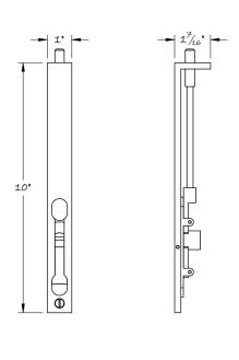
Lowe Hardware's No. 4066 flush bolt is designed to make pocket doors steadfast while under way, either in the open or closed position. The piece can also be used on swinging door pairs, where the bolt is usually installed top and bottom on the inactive door.
